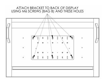
Figure 8. Display with 400mm x 200mm Hole Pattern
